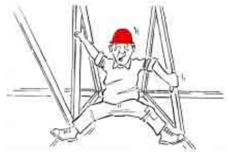
TRUSSES DO NEED BRACING
